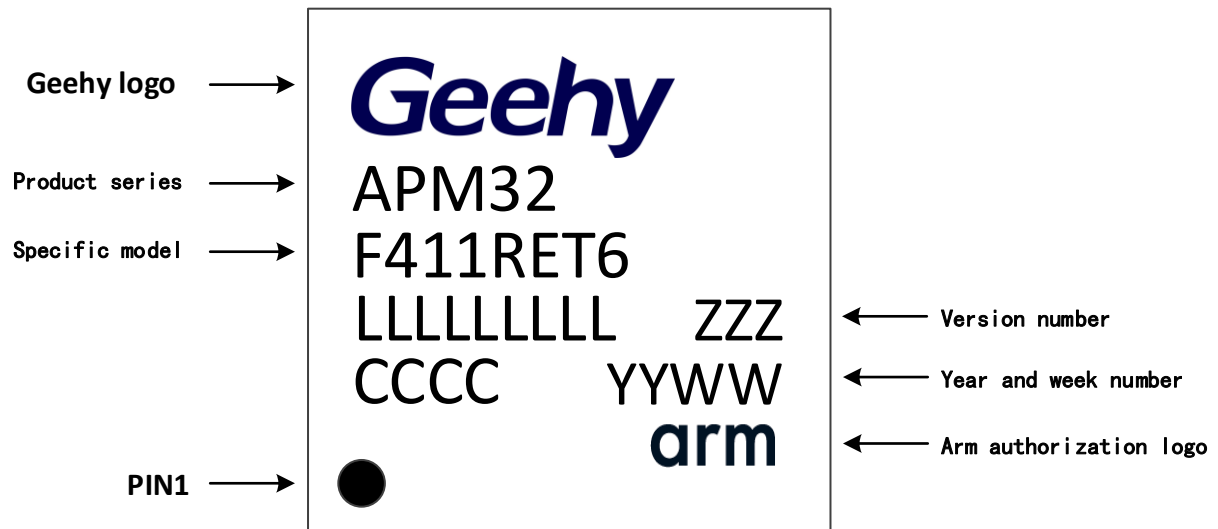
Figure 22 LQFP64 - 64 Pins, 10 x 10mm Diagram
