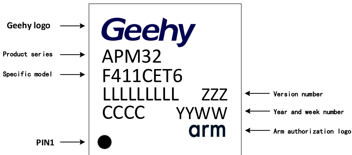
Figure 25 LQFP48 - 48 Pins, 10 x 10mm Diagram
